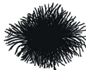
Pointed needle-like primary crystallites form a fibrous coating on the particles of the special coating, allowing to actively displace the water.
