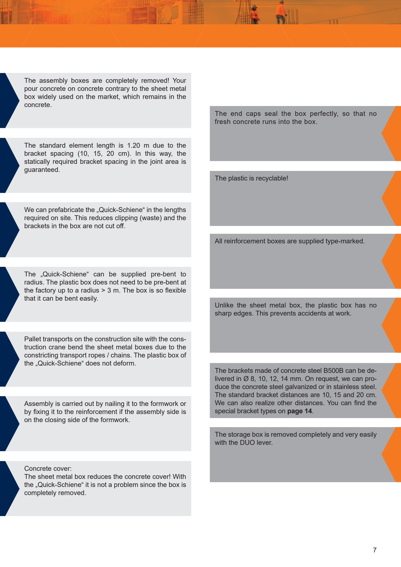
The assembly boxes are completely removed! Your pour concrete on concrete contrary to the sheet metal box widely used on the market, which remains in the concrete.
